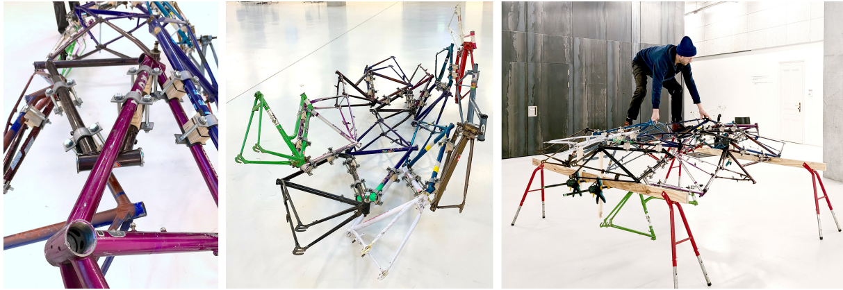
Figure 5: Curved configuration in detail (left), and in horizontal setup for dynamic load bearing assessment (right)
