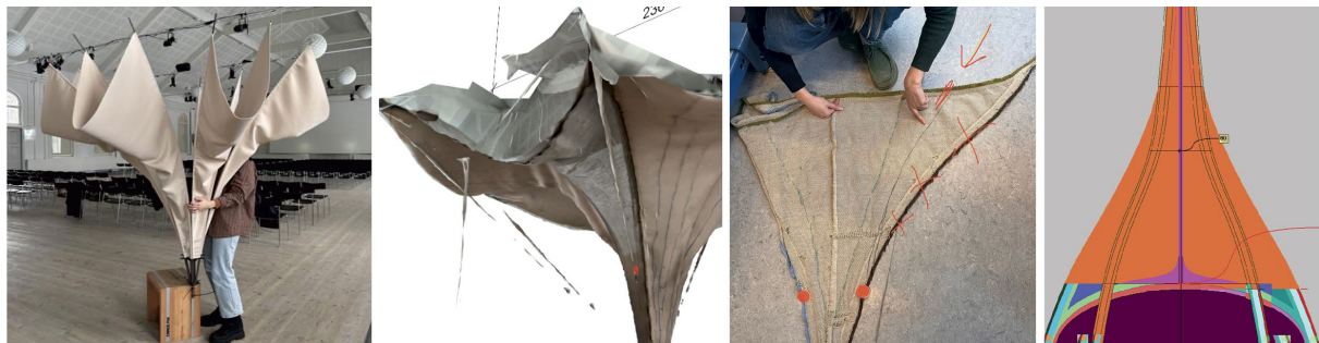
Figure 9: Incremental prototyping method for the CNC-knit textiles and the hybrid system of HempHalo with active bending rods
