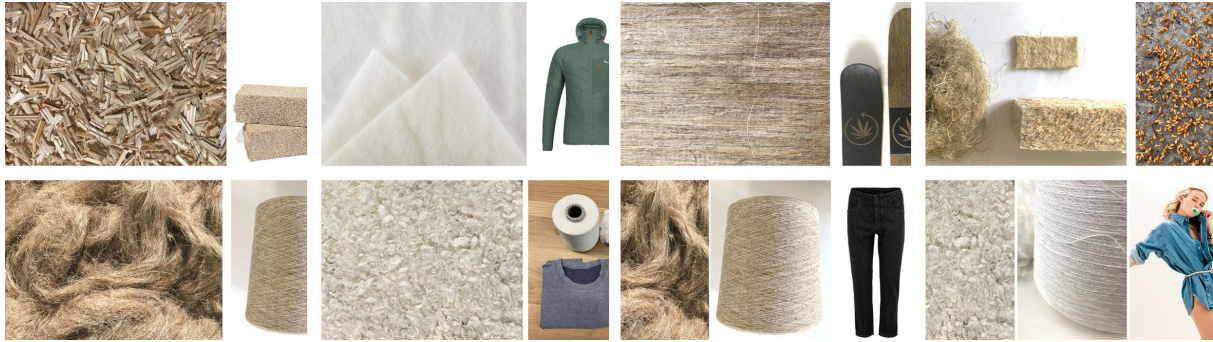
Figure 3: State of the art in short hemp fiber applications as fillers, insulation jacket lining (Salewa/Imbotex), stitched fibre mats for composite applications (FUSE, SPURart), needle punched felt for geotextiles (Seidemann), hemp blended yarns for garment (Candiani, Lenzing)
