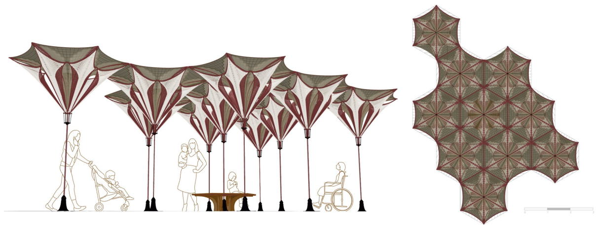
Figure 2: Vision of the double-layer canopy system using 100% hemp-based CNC-knitted differentiated membrane and hemp pultruded rods
