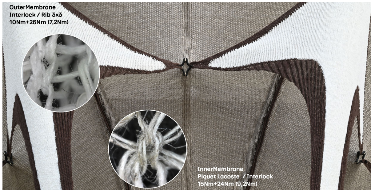
Figure 6: Two Textile Membrane Layers of the HempHalo
