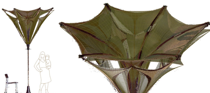
Figure 10: 3D Scanning documentation of the Final Prototype Assembly of HempHalo for further evaluation of the tolerances
