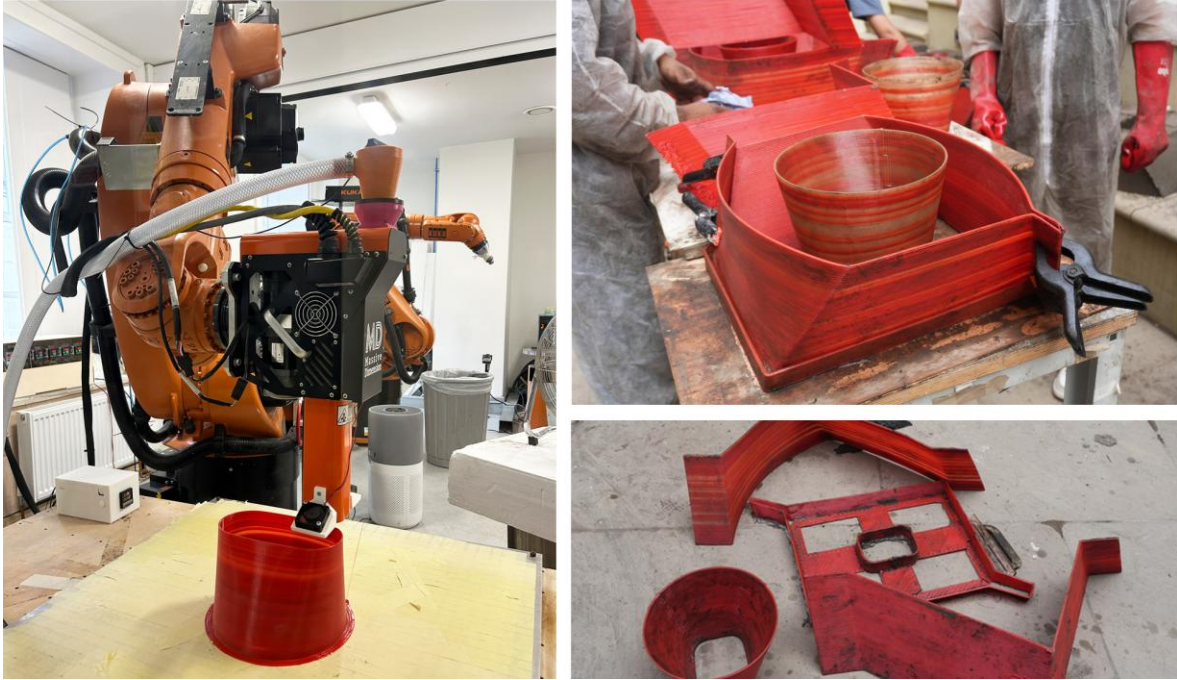
Figure 5. Robotic 3D printing of reusable formworks utilized for the concrete casting of osteomorphic interlocking blocks.
