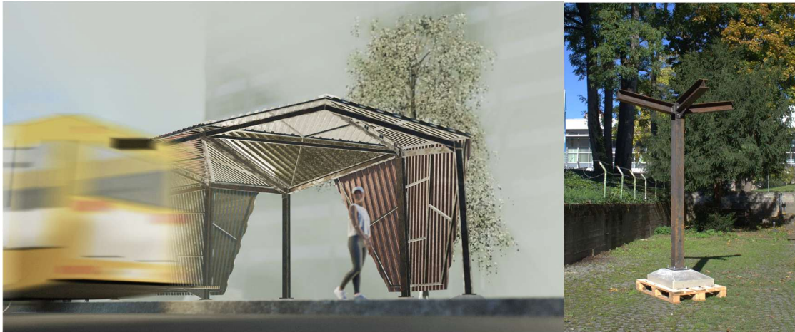
Figure 5: Rendering of the design developed based on the proposed workflow (left) and the portion of the design realized from reclaimed steel beams as a full-scale demonstrator. (right)
