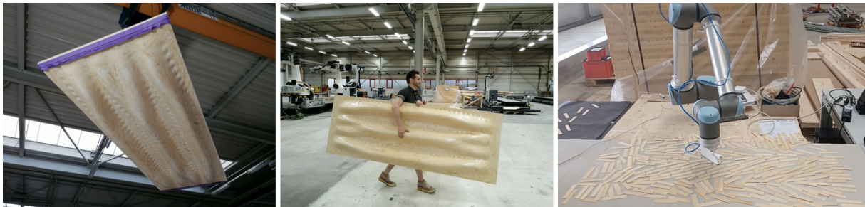
Figure 13: Fabricated slab prototype (left) and robotic strand layup test.
