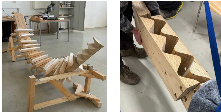
Figure 5: Left: Gluing a segment using wooden clamps along each ruling line in the correct direction and position to allow for the twist; Right: Assembly of the vertical scarf joint
