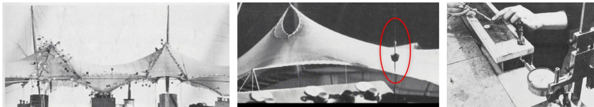
Figure 3: a) polyester fabric net; b) surveying at the IL measuring table (plumb line in red circle); c) applying the preload [p.283 in [5]; p.283 in [5]; p.284 in [5]]
